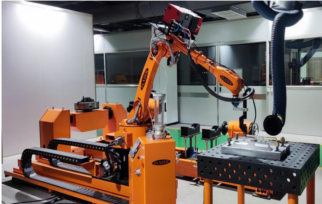
FIGURE 10 AN INSTALLATION FOR 3D PRINTING OF LARGE-SCALE PARTS USING HYBRID PLASMA TRANSFERRED ARC SURFACING WITH WIRE AND POWDER, DEVELOPED AT THE E.O. PATON ELECTRIC WELDING INSTITUTE
